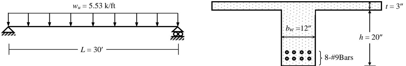
Given  $f'_c = 3$  ksi,  $f_y = 60$  ksi, and beam dimensions of  $b_w = 12''$  and  $h = 20''$
