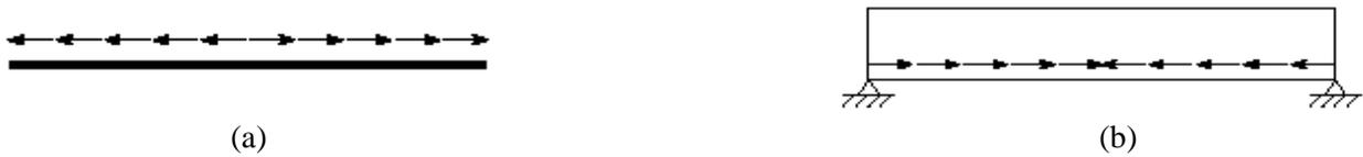
Fig. 10.2: Bond forces on steel and concrete (Nilson)
