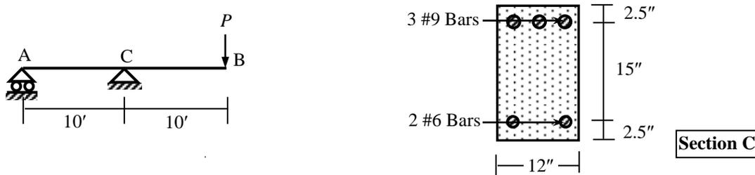
4. Answer Question 3 assuming Section C to have cracked but  $f_c$ ,  $f_s$  and  $f_s'$  are to remain within the allowable limits.
