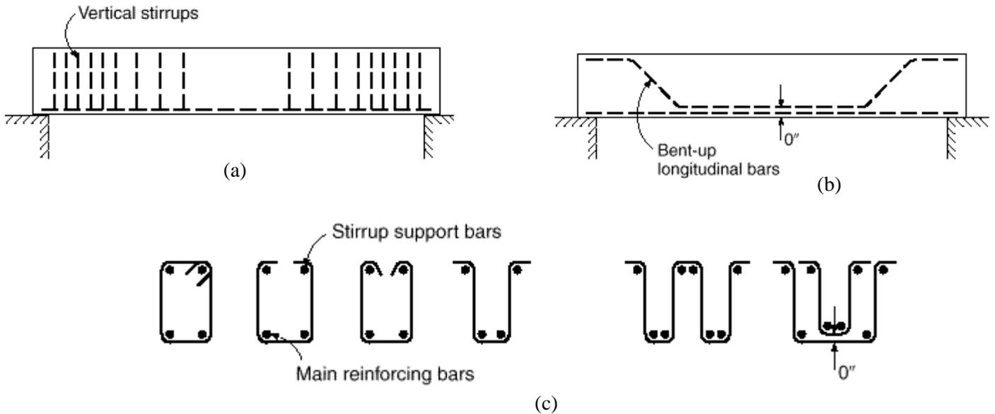
Fig. 8.5: (a) Vertical stirrups, (b) Bent-up longitudinal bars, (c) Various forms of stirrups (Nilson)
