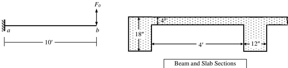
3. Use the WSD method to design the section  $c$  of the fixed-ended beam  $ab$  shown in the figures below if (i)  $P = 5$  kips, (ii)  $P = 10$  kips. Exclude the weights from the slab and beam [Given:  $f_c' = 3$  ksi,  $f_s = 18$  ksi].
