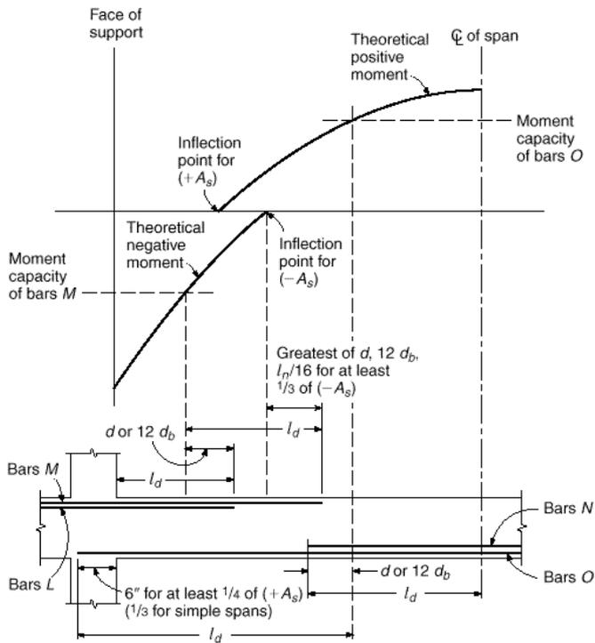
Fig. 10.9: Bar cutoff requirements of ACI Code (Nilson)
