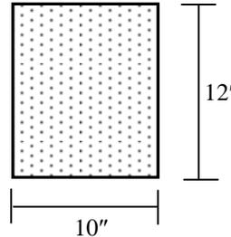
3. Use the WSD method to design section B of the cantilever RC beam AB shown in the figure below as a singly reinforced beam (i) excluding its self-weight, (ii) including its self-weight [Given:  $f_c' = 4$  ksi,  $f_s = 24$  ksi].
