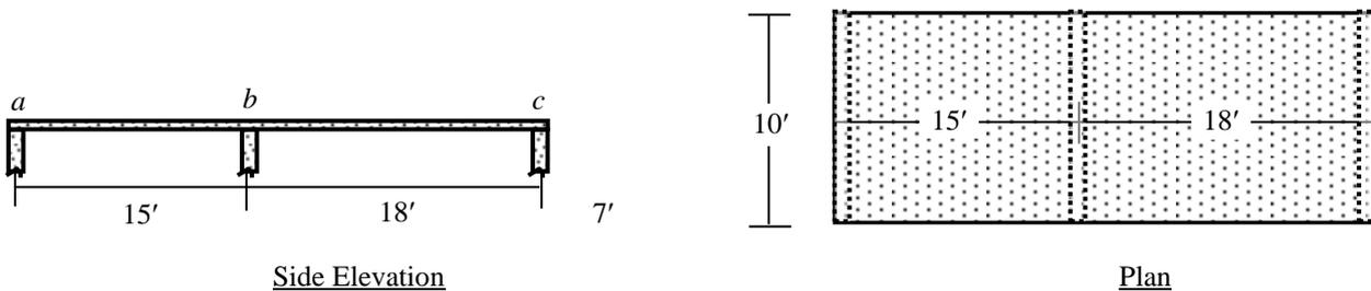
5. Calculate the live load that can be carried by the slab shown below (carrying  $FF = 30$  psf,  $RW = 50$  psf), if it is reinforced (longitudinally) as shown below. Also show its reinforcements in the transverse direction [Use ACI moment coefficients, with  $f_c' = 4$  ksi,  $f_y = 60$  ksi].
