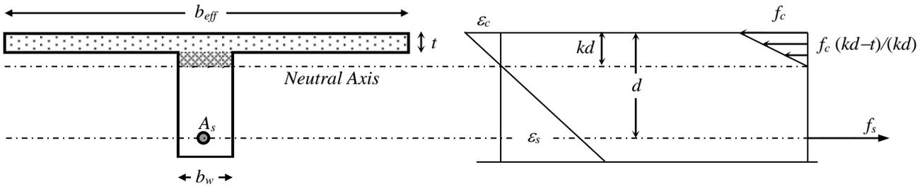
Fig. 7.2: Working Strain and Stress distribution in T-Beam
