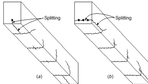
Fig. 10.3: Splitting of Concrete along Reinforcement (Nilson)
