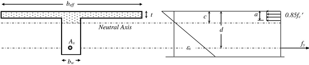
Fig. 7.3: Ultimate Strain and Stress distribution in T-Beam
