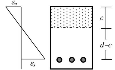
Fig. 6.1: Strains at Compression Failure
