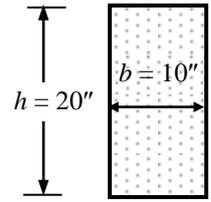
In WSD,  $v_{cw} = 1.1\sqrt{f_c'} = 60.2$  psi,  $v_{cw1} = 3\sqrt{f_c'} = 164.3$  psi,  $v_{cw2} = 5\sqrt{f_c'} = 273.9$  psi
