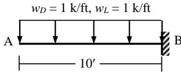
Using load factors 1.4 for dead load and 1.7 for live load, the ultimate load,  $w_u = 1.4 \times 1 + 1.7 \times 1 = 3.1$  k/ft
