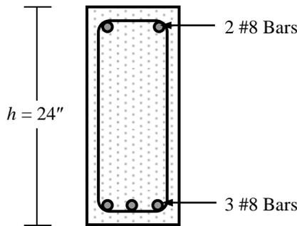
The allowable moment in the section after cutting off 2 bottom bars can be calculated by analyzing the section.
