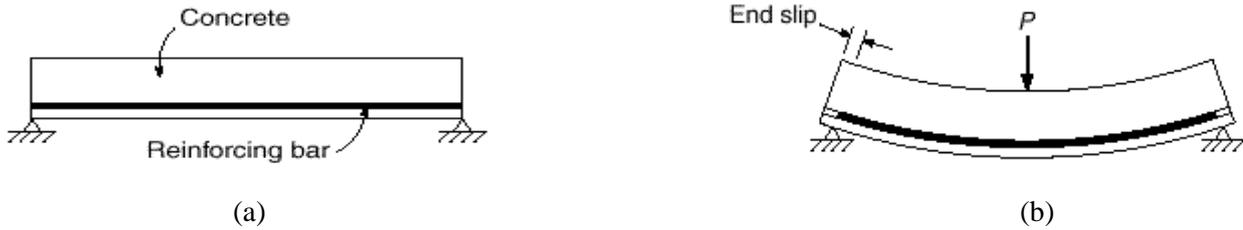
Fig. 10.1: Beam before and after loading (Nilson)
