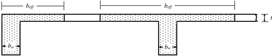
Fig. 7.1: Effective Widths of L- and T-Beams
