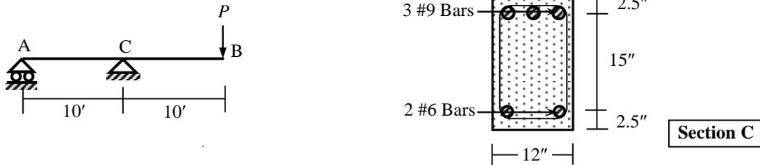
3. Use the USD to calculate the maximum allowable live load  $w$  k/ft on the RC cantilever beam (with sections B) shown below [Given:  $f_c' = 3$  ksi,  $f_y = 40$  ksi].
