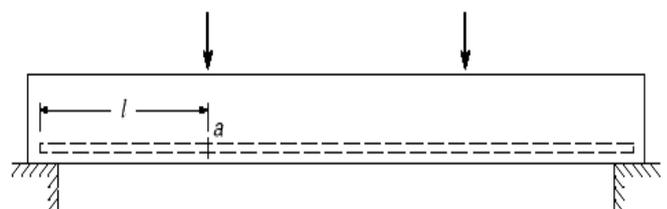
Fig. 10.5: Development Length of Reinforcing Bar (Nilson)
