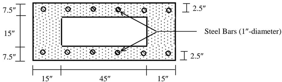
6. In Question 3, calculate the ultimate value of  $P$  in beam AB if columns A and C are both made of (16"×16") RC sections, as shown in the figure below. Also calculate the stresses in concrete and steel when the section is subjected to one-half its ultimate load [Given:  $f_c' = 4$  ksi,  $f_y = 50$  ksi].
