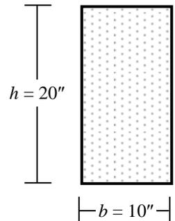
Given beam dimensions of  $b = 10''$  and  $h = 20''$
