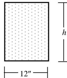
6. Design the RC beam  $abcd$  loaded as shown below (in addition to self weight) for the maximum positive and negative moments, if it has a (12" × 16") cross-section shown alongside [Given:  $f_c' = 3$  ksi,  $f_s = 20$  ksi].
