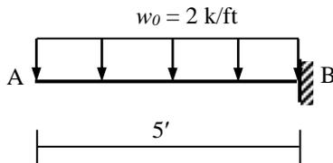
4. Design the cantilever beam shown in Question 3 if it has a (10" × 12") cross-section shown in Question 2.
