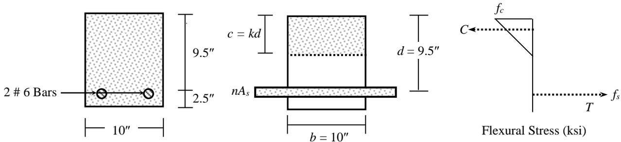
Fig. 3.2: (i) Cross-section, (ii) Equivalent Uncracked Section, (iii) Flexural Stresses
