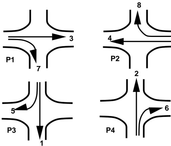
Figure 41:3: One way of providing four phase signals
