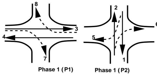
Figure 41:2: Two phase signal
