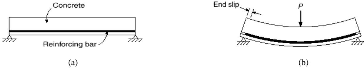
Fig. 10.1: Beam before and after loading (Nilson)
