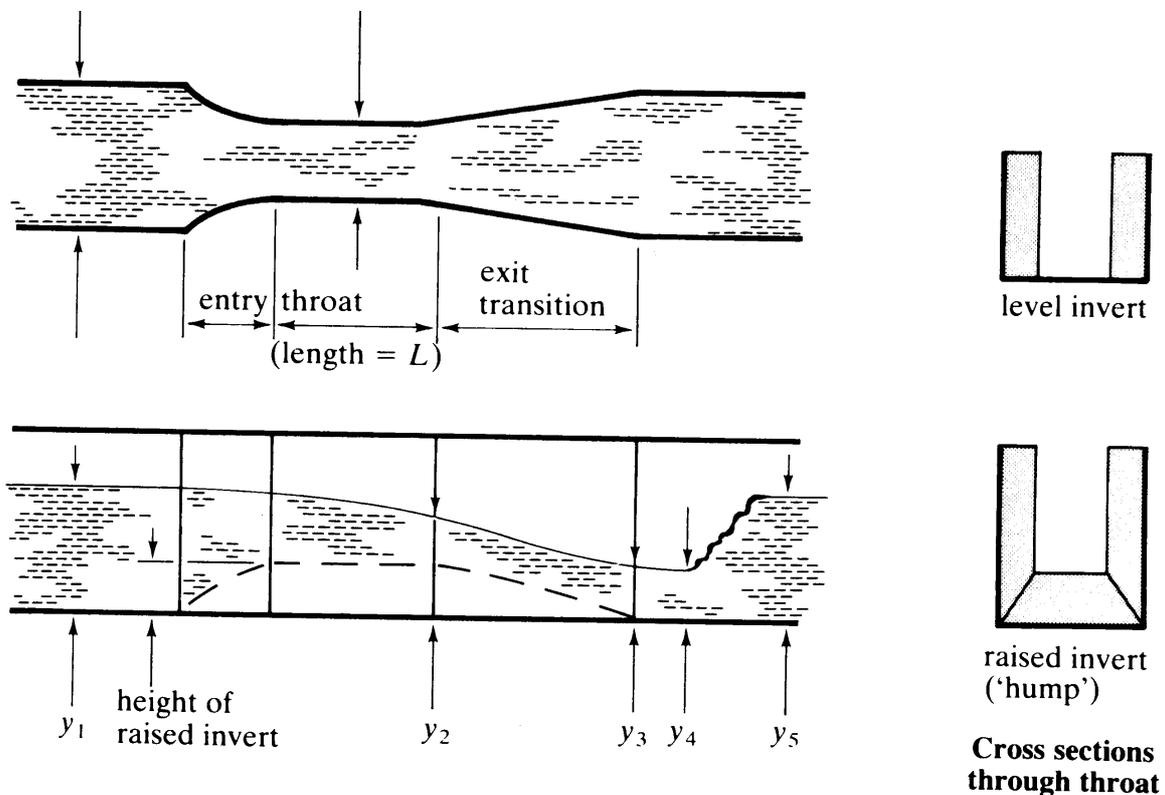
Figure of section through a Venturi flume
