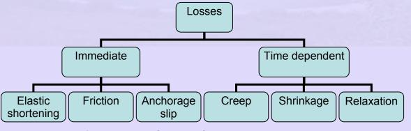
Figure 2-1.3 Causes of the various losses in prestress
