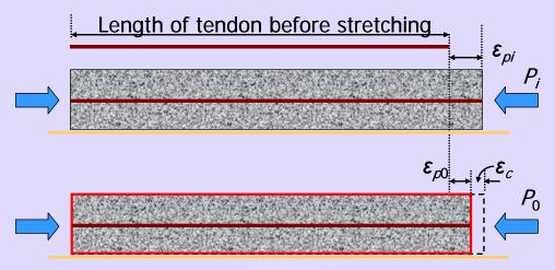
Figure 2-1.5 Strain variables in elastic shortening
