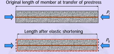
Figure 2-1.4 Elastic shortening of a pre-tensioned axial member
