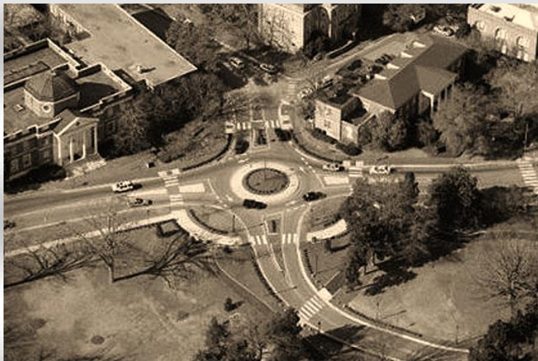
Figure 10.13 Typical layout of a single lane modern roundabout. Source: Kimley-Horn and Associates, Inc.
