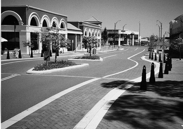
Figure 10.17 A mid block crossing with a flush curb in New Zealand. Pedestrians are separated from passing vehicles with bollards. Source: Community, Design + Architecture.
