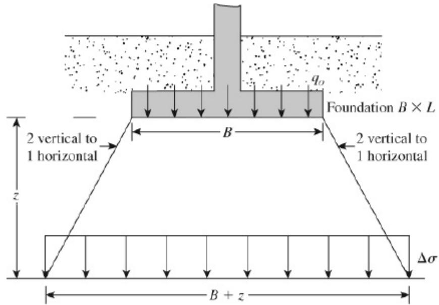
Fig 6.4 Two is to one method
