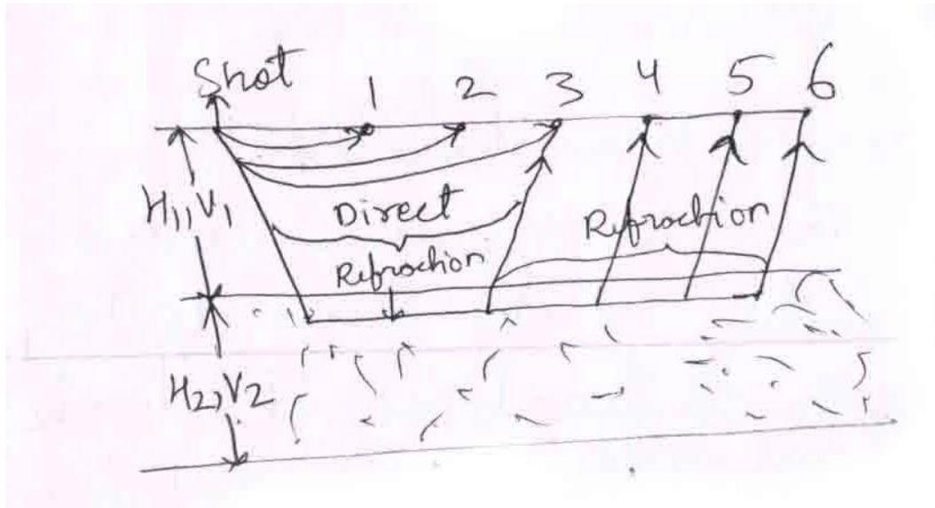
Fig. 15.2 Travel of primary and refracted waves
