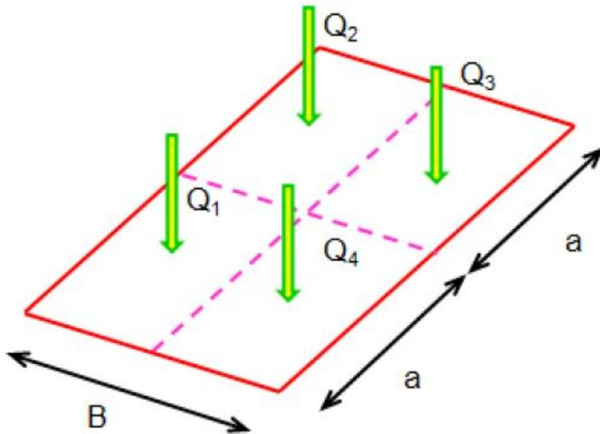
Fig 6.3 Equivalent point load method
