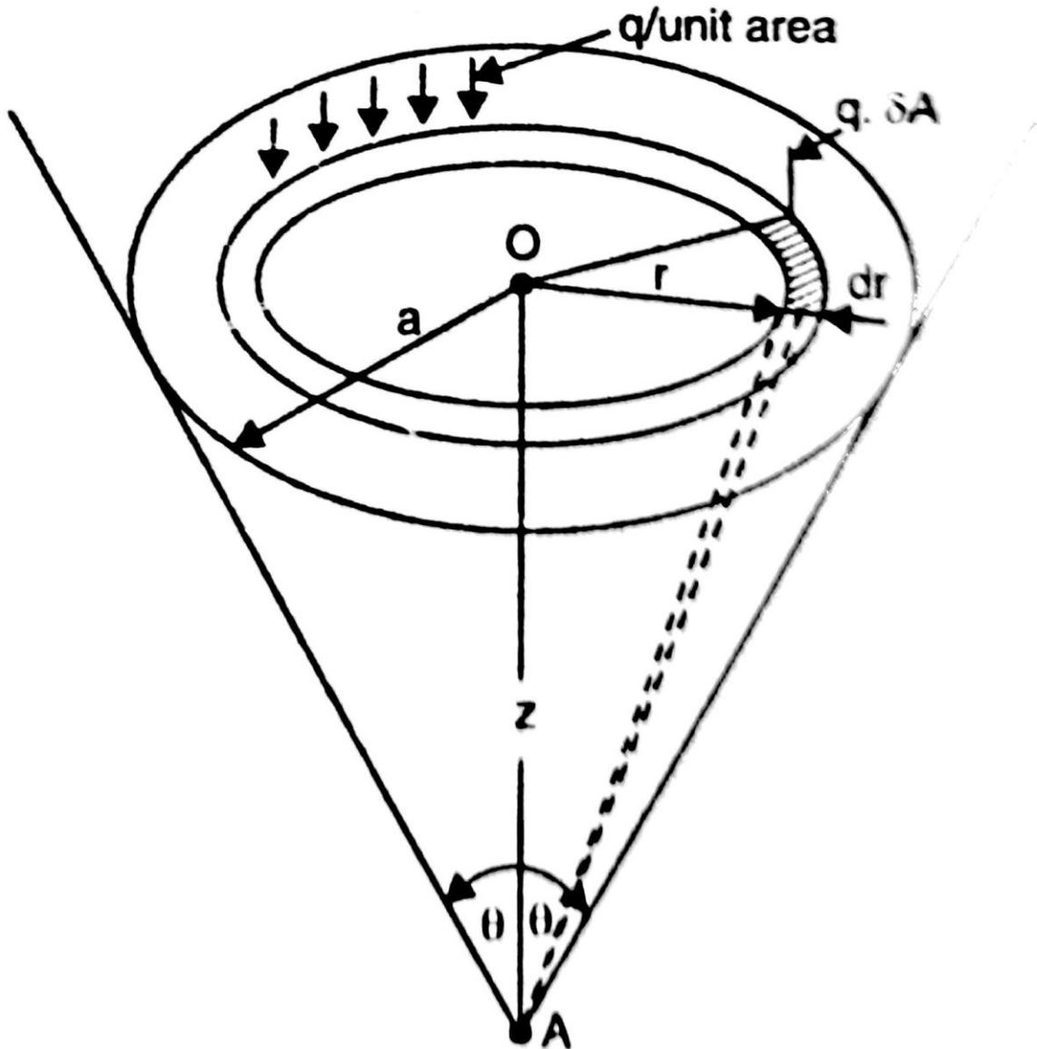
Fig 5.2 Uniform load over circular area.
