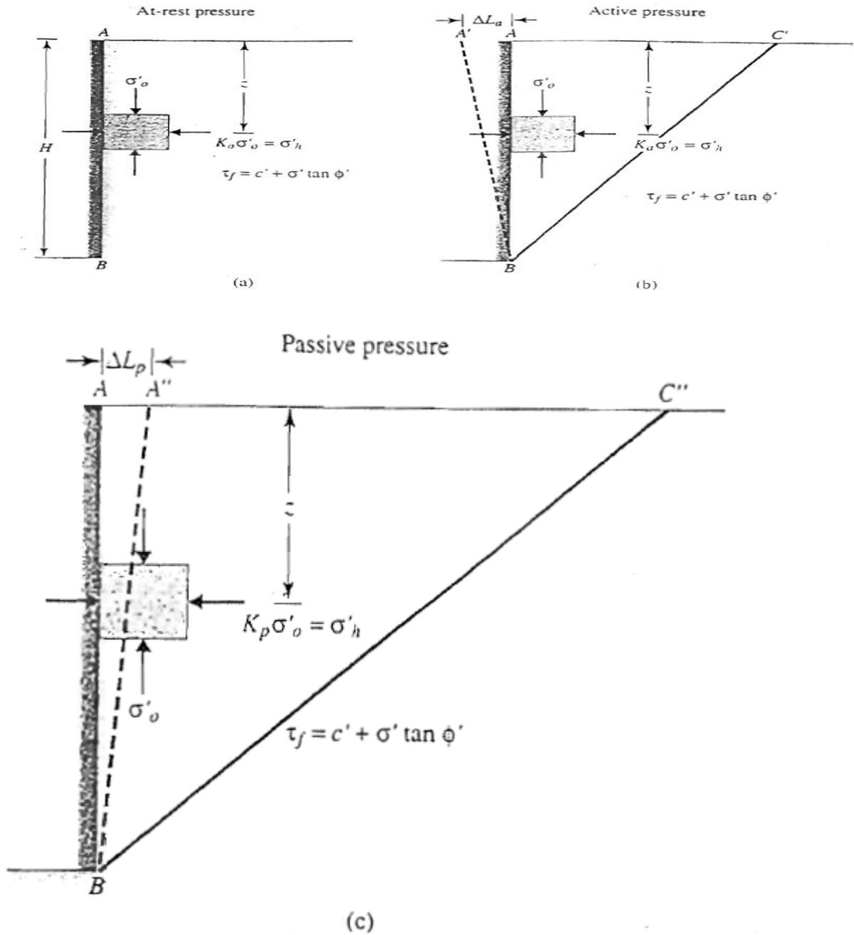
Fig. 7.3 Definition of at – rest, and passive pressures (Note : Wall AB is frictionless)
