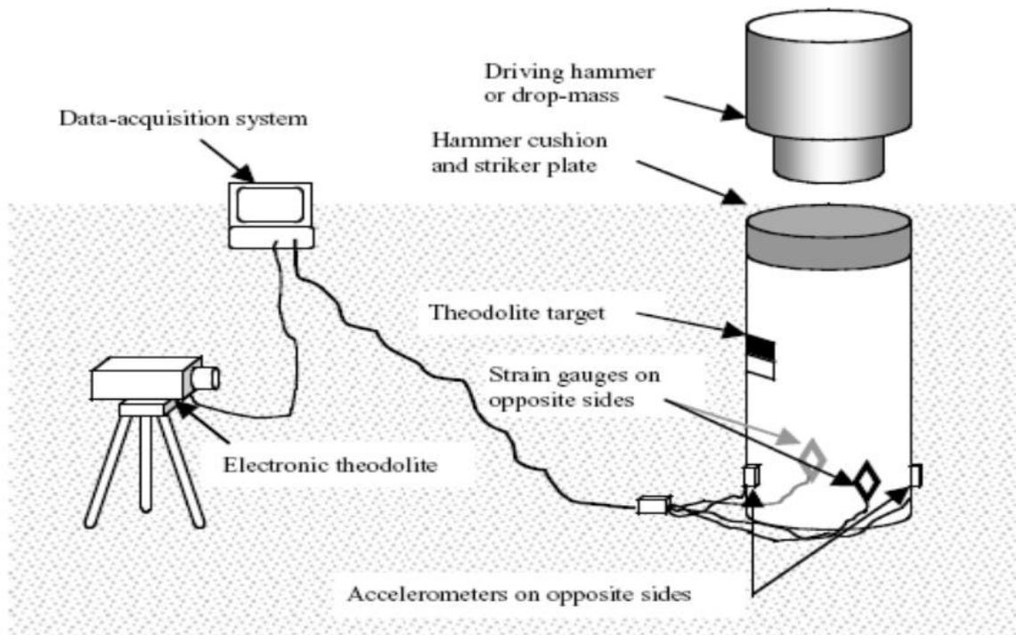
**Figure 40.1:** Schematic of SIMBAT Instrumentation
