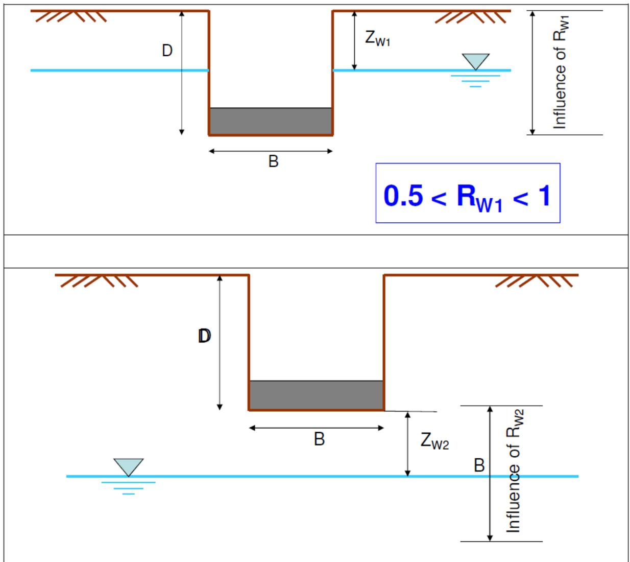
Fig. 28.1 Effect of water table on bearing capacity.
