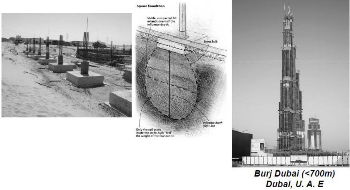
**Fig. 1.5** Subsurface stresses in soils are increased by foundation loads
