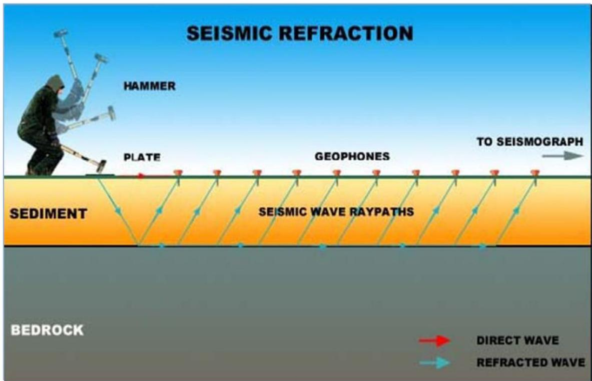
Fig.24.2 Seismic refraction method
