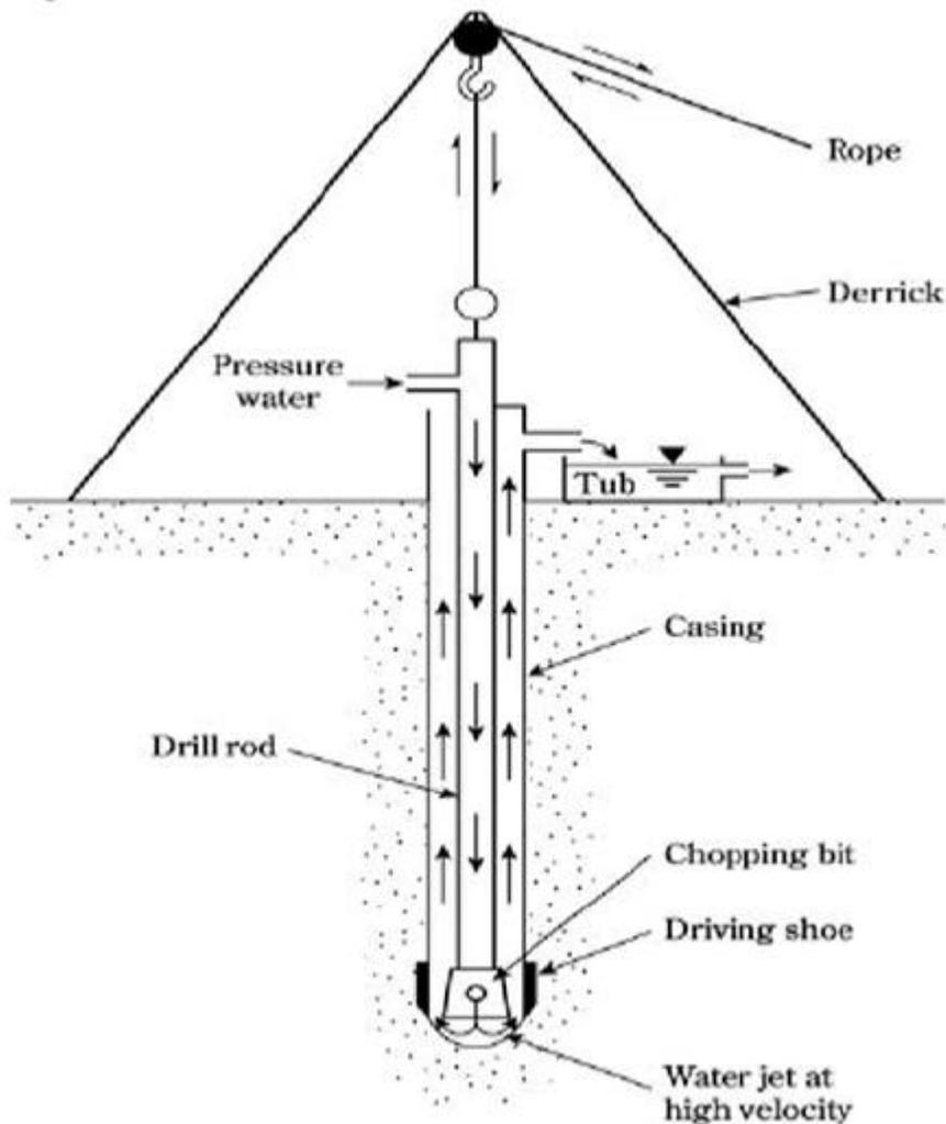
**Fig.18. 1** Wash Boring set up
