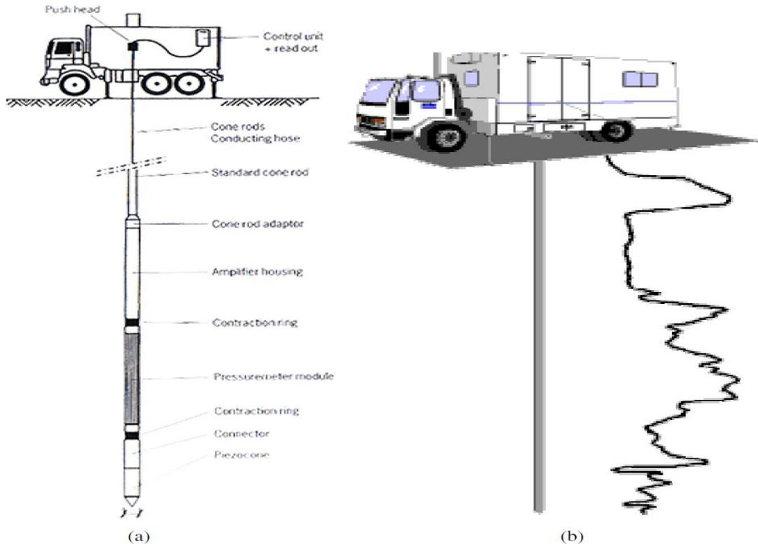
**Fig.22.1 Cone penetration set up**
