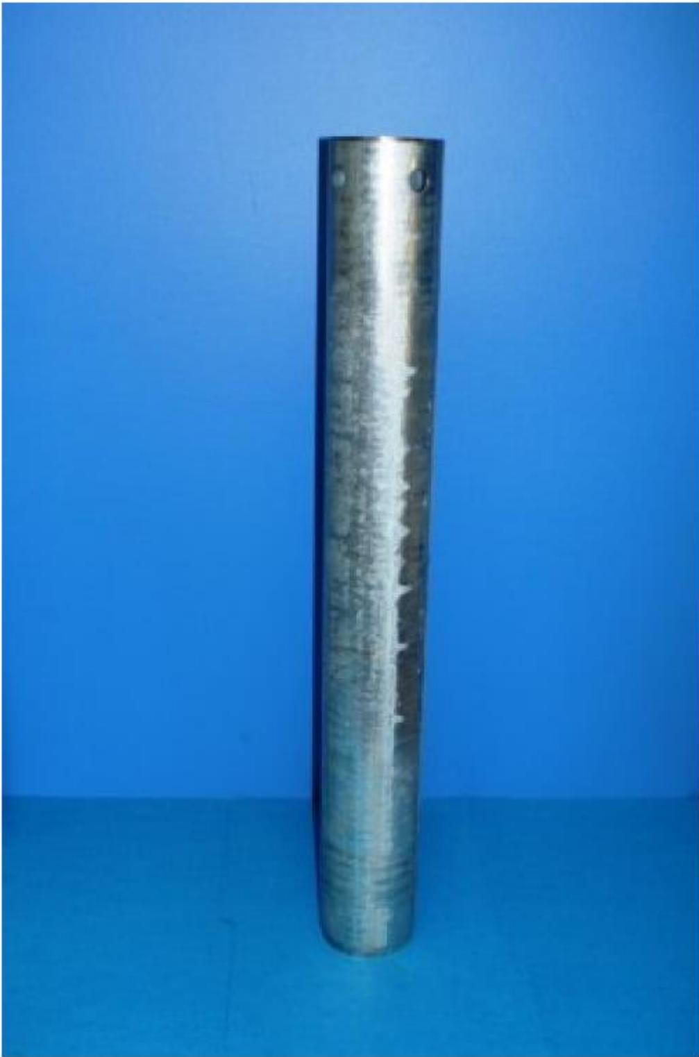
**Plate 19.4 Shelby tube sampler**
