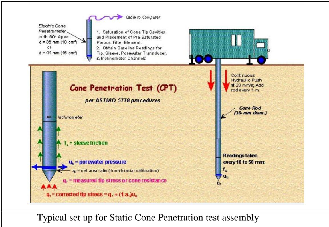
Typical set up for Static Cone Penetration test assembly
