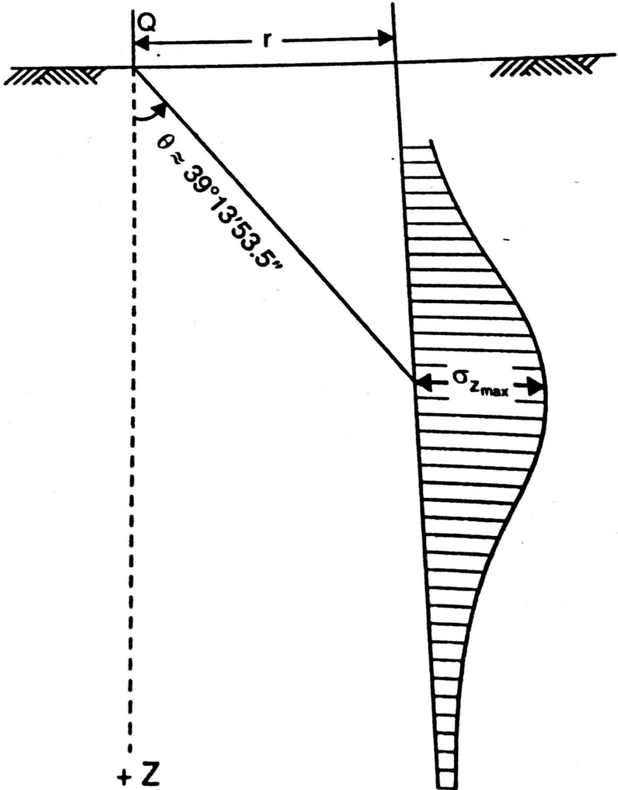
**Fig. 3.3** Vertical stress distribution along a vertical line at radial distance ' $r$ '
