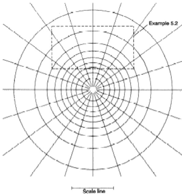
Fig 6.2 *vertical stress increase at z*
