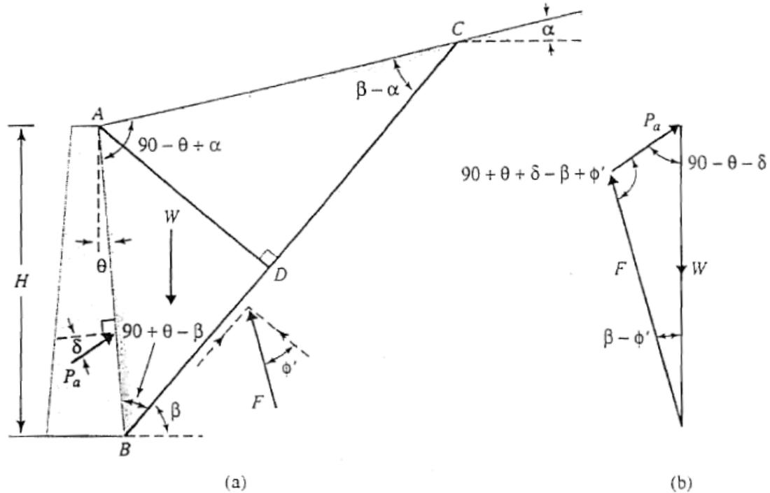
Fig. 10.1 Coulomb's active pressure (a) Trial Failure wedge (b) Force polygon
