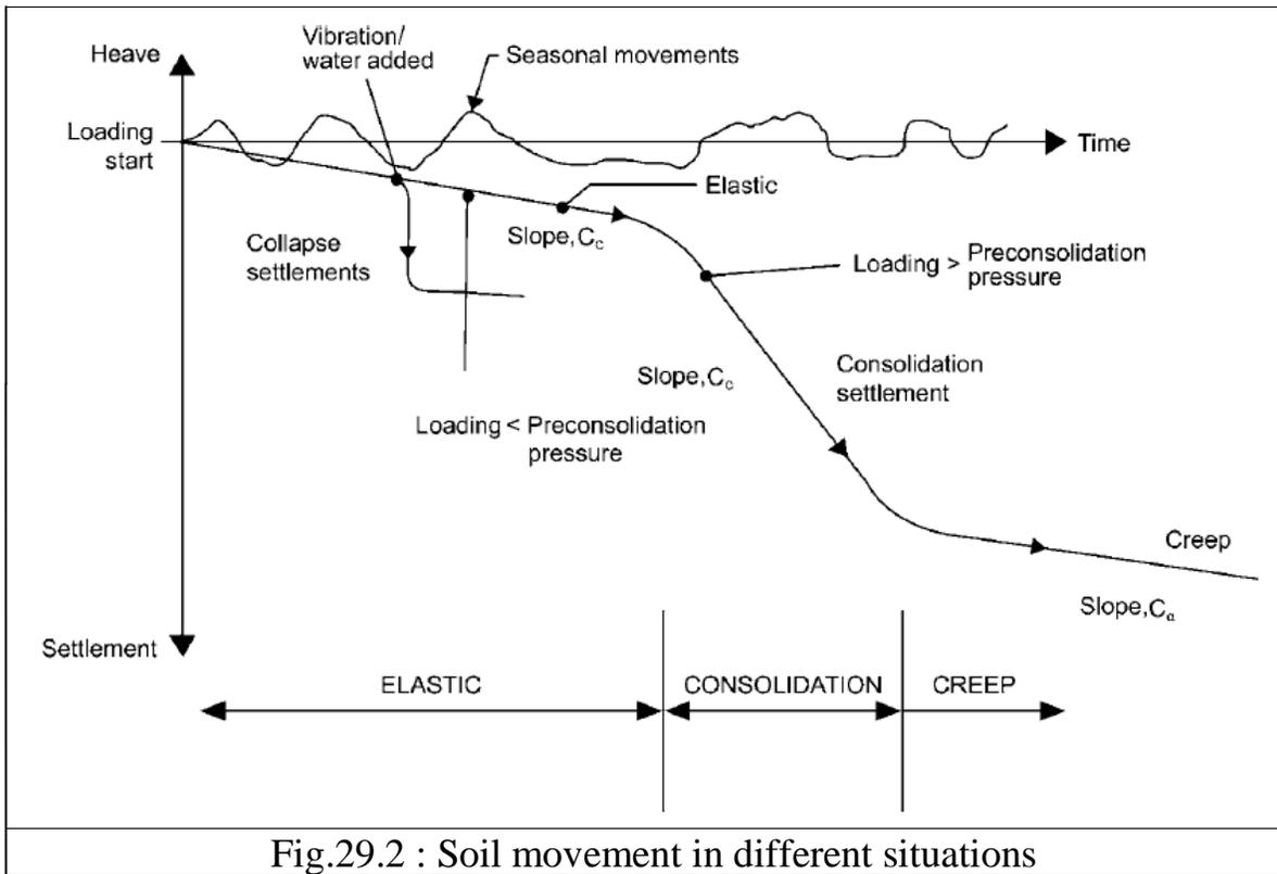
Fig.29.2 : Soil movement in different situations
