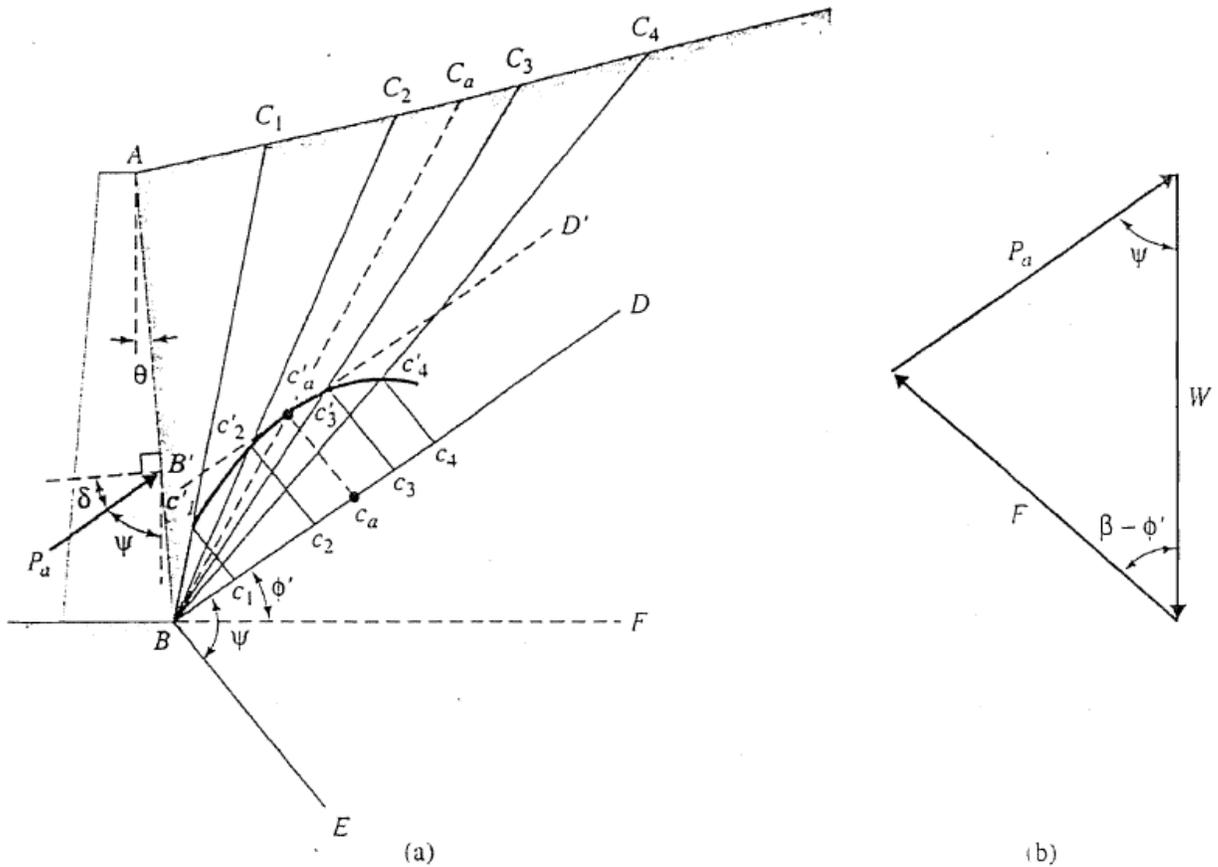
Fig. 10.2 Culmann's solution for active earth pressure.
