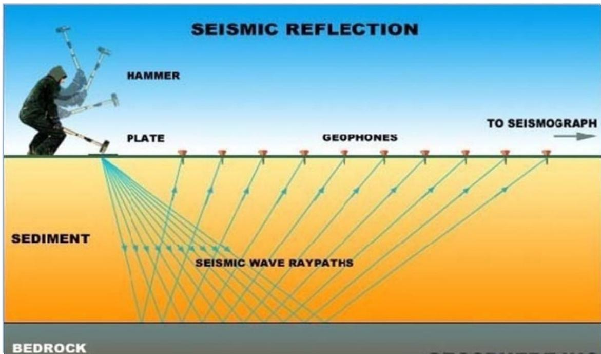
Fig. 23.1 Seismic Reflection method
