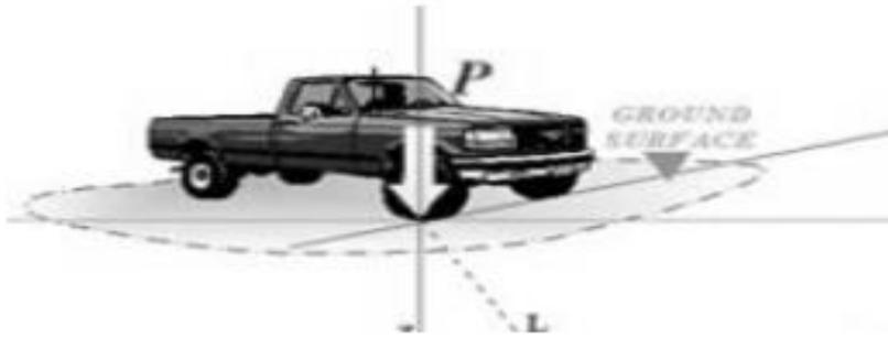
**Fig. 2.3 Subsurface stress increment due to a point load**
