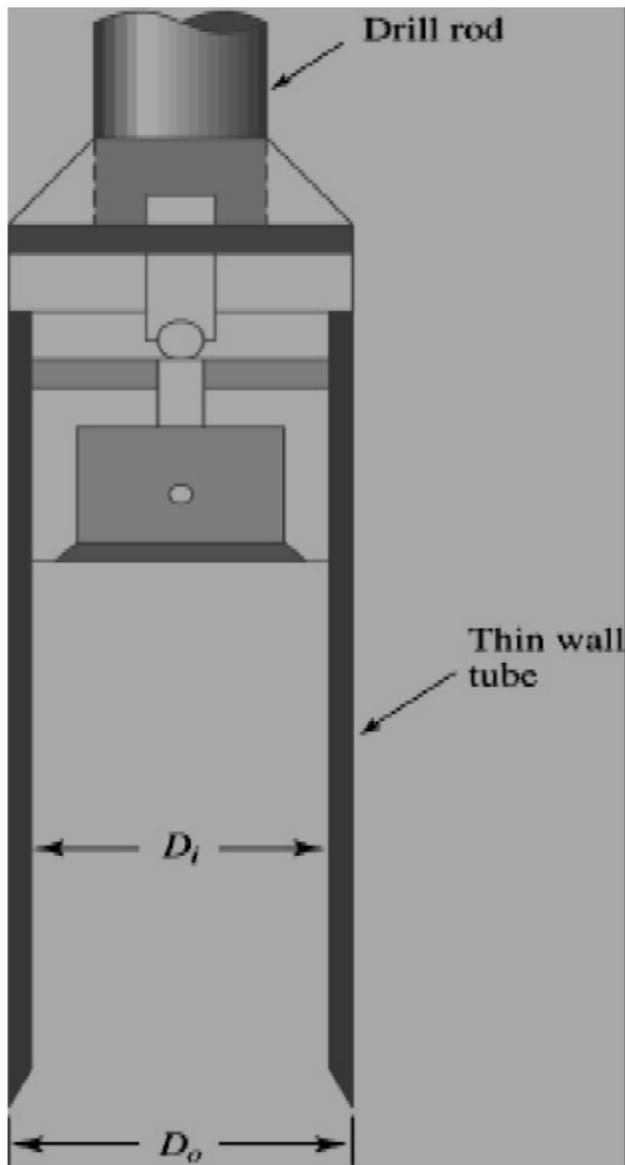
Fig.19.3 Shelby tube sampler
