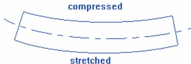
Bending stress is distributed through a beam as seen in the diagram below:
