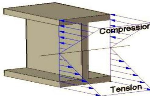
So, in reality, bending stresses are tensile or compressive stresses in the beam! A simply-supported beam always has tensile stresses at the bottom of the beam and compressive stresses at the top of the beam.
