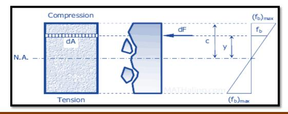
Considering a differential area dA at a distance y from N.A., the force acting over the area is
