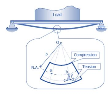
Consider a fiber at a distance y from the neutral axis, because of the beam's curvature, as the effect of bending moment, the fiber is stretched by an amount of cd. Since the curvature of the beam is very small, bcd and Oba are considered as similar triangles. The strain on this fiber is
