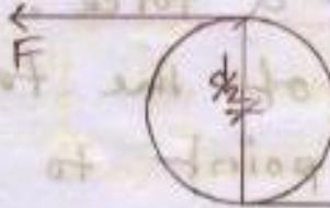
**Torque or turning moment:** Torque is moment of a force or forces about an axis of rotation.
