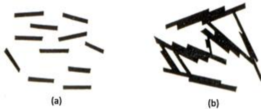
Figure 1.17 (a) Dispersion and (b) flocculation of clay
