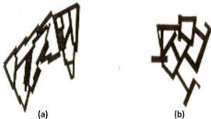
Figure 1.18 (a) salt and (b) non-salt flocculation of clay particles. (after T. W. Lamber, Compacted Clay: Structure , Trans. ASCE, vol. 125, 1960)
