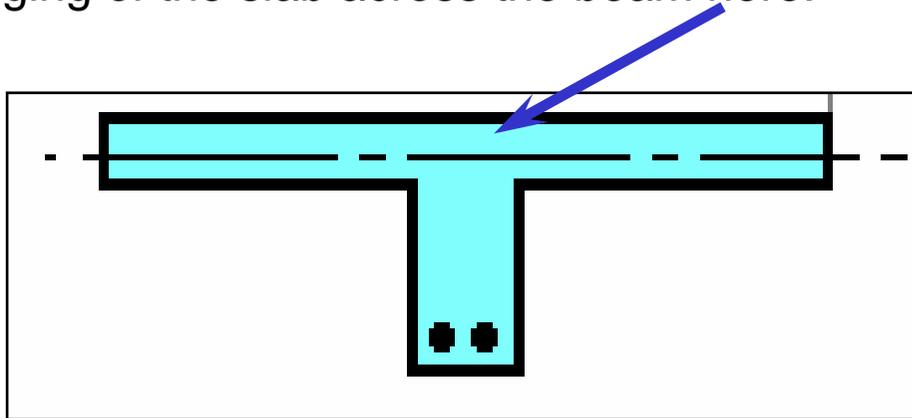
**The concrete is subjected to a two-dimensional stress state. At first glance, this may appear to be a problem. However, this is not the case.**
