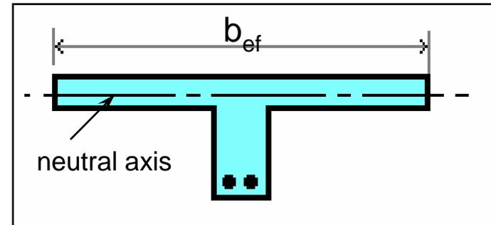
So a T-beam or an L-beam can be designed just as for a rectangular beam, except for the following considerations:
