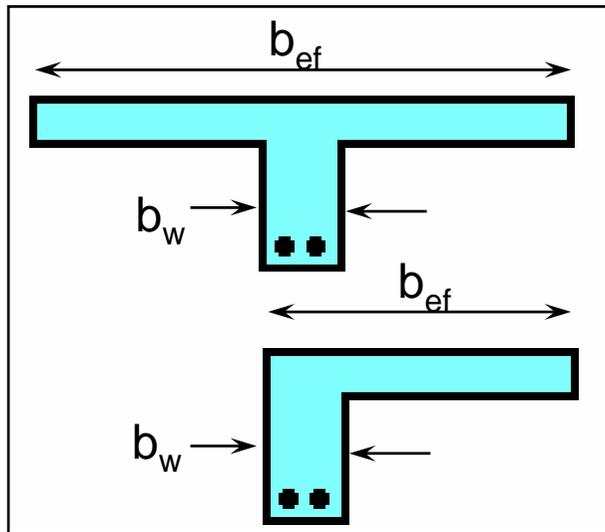
The width of flange clearly cannot exceed half the distance to the next adjacent beam (otherwise we'd be double-counting).
