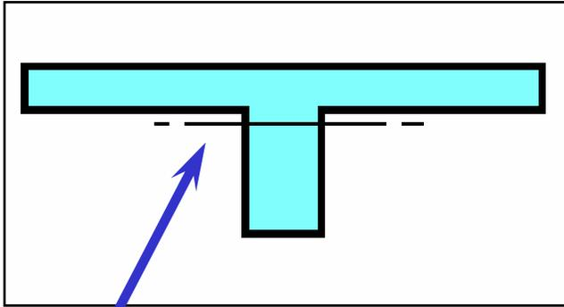
Note that the neutral axis of the *uncracked* section may be below (as shown) or within the flange.
