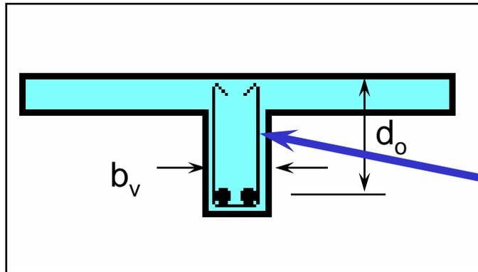
Vertical shear action is carried by the web, which includes the common web/flange area.
