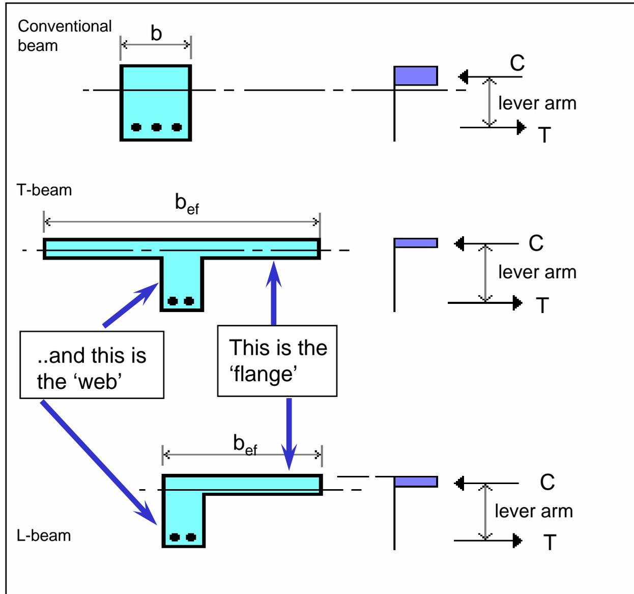
Since T-beams and L-beams have a greater effective width of compression flange ( $b_{ef} > b$ ), a greater lever arm is available.
