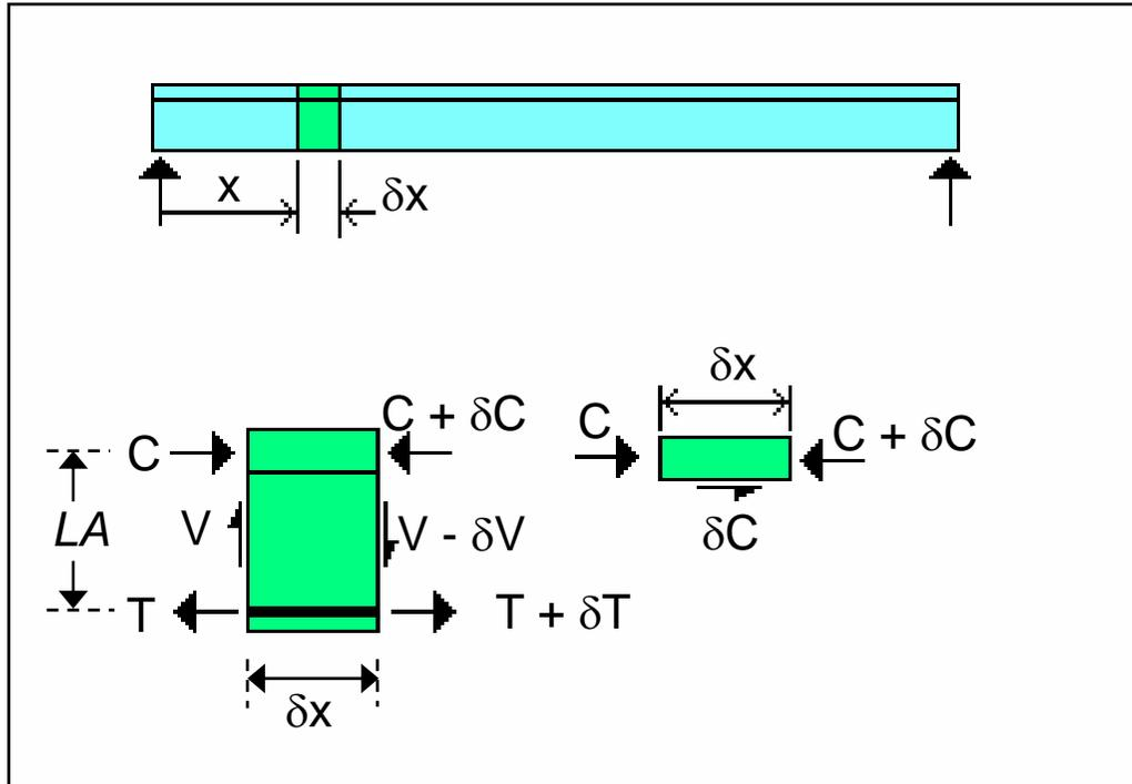
Over distance  $\delta x$ , a horizontal shear force  $\delta C$  must be provided to ensure integrity of the beam.
