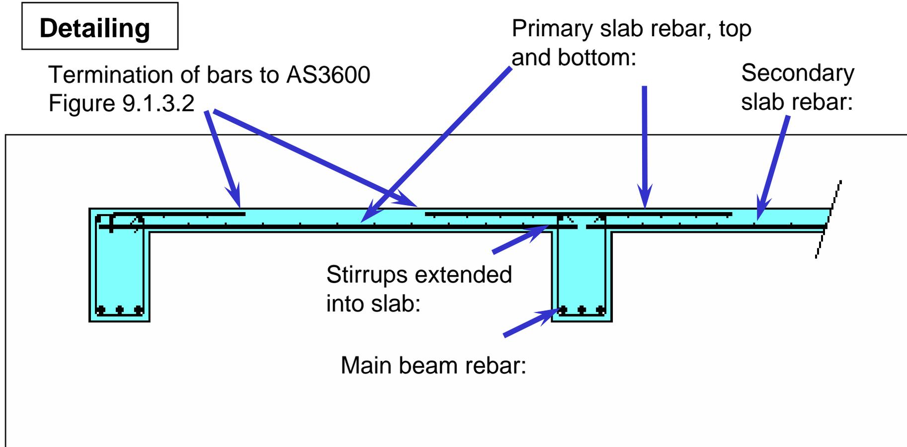
The slab is designed as a one-way, continuous slab, spanning across the beam supports.
