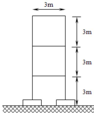
Figure 6.17: Frame to be analyzed by Seismic soil-structure interaction analysis.
