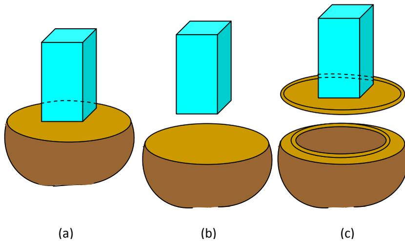
Figure 6.14: Seismic soil-structure interaction with substructure method: (a) SDOF system resting on a half space; (b) modeling superstructure and soil medium separately; (c) some portion of the soil is included in the superstructure model.
