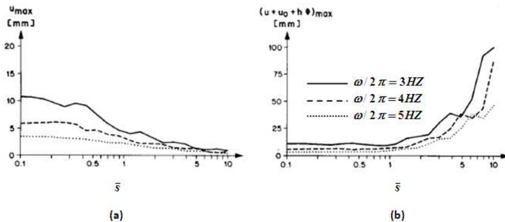
Figure 6.11: Response of equivalent SDOF system to artificial time history, considering SSI ( $\bar{h} = 1, \bar{m} = 3, \nu = 0.33, \xi = 0.025, \xi_s = 0.05$ ): (a) maximum structural displacement; (b) maximum displacement of mass relative to free field (Wolf, 1985).
