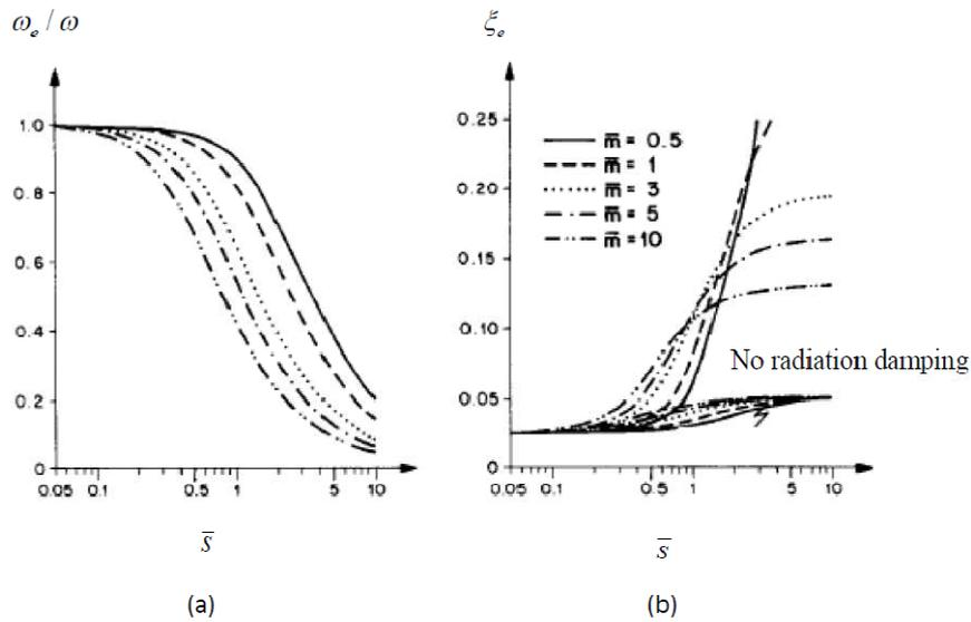
Figure 6.10: Effect of stiffness ratio and mass ratio on (a) natural frequency and (b) damping ratio of soil-structure system ( $\bar{h} = 1, \nu = 0.33, \xi = 0.025, \xi_s = 0.05$ ) (Wolf, 1985).
