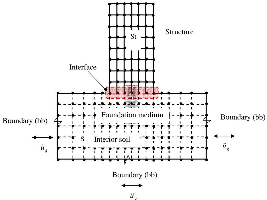
Figure 6.12: Finite element model of soil-structure system for direct method of analysis.
