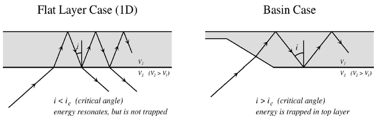
Figure 6.2: Schematic diagram showing that seismic waves entering a sedimentary layer from below will resonate within the layer but escape if the layer is flat (left) but become trapped in the layer if it has varying thickness and the wave enters the layer through its edge (right) (After Grave, 1998).
