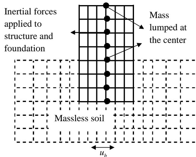
Figure 6.8: Inertial interaction analysis
