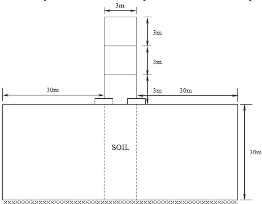
Figure 6.19: ABAQUS model of structure with soil.
