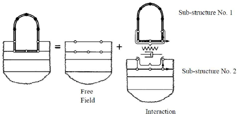
Figure 6.13: Seismic soil-structure interaction with substructure method. (Wolf, 1985)
