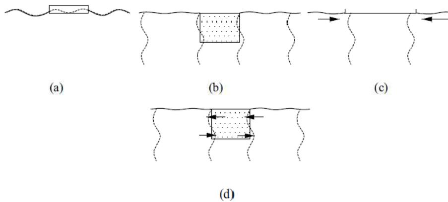
Figure 6.5: Kinematic interaction: (a) vertical motion modified; (b) horizontal motion modified; (c) incoherent ground motion prevented; and (d) rocking motion introduced (Datta, 2010).
