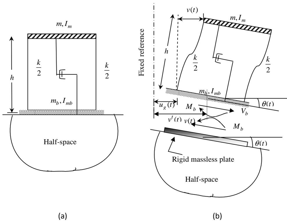
Figure 6.15: Seismic soil-structure interaction analysis using substructure method for SDOF system.
