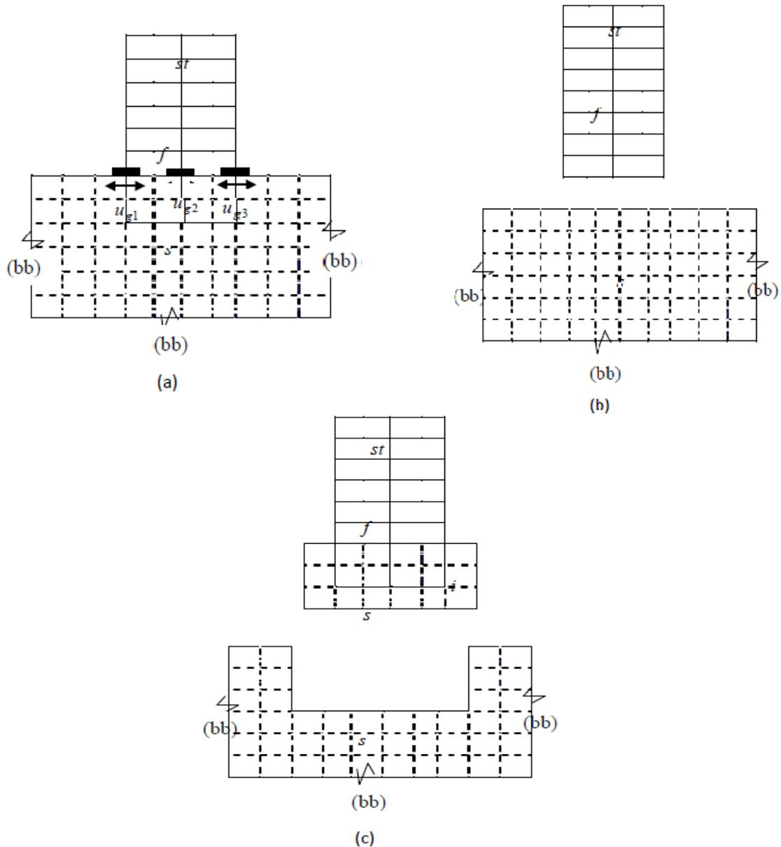
Figure 6.16: Seismic SSI with substructure method: (a) MDOF system with multi-support excitation; (b) modeling superstructure (substructure no. 1) and soil medium (i.e. substructure no. 2) separately; (c) some portion of the soil is included in the superstructure model referred as substructure no.1 and remaining soil as substructure no. 2.
