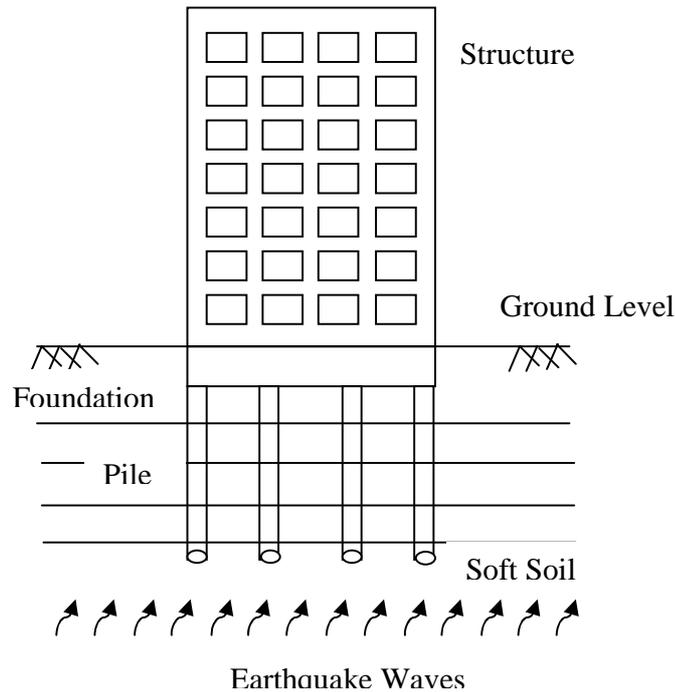
Figure 6.1: Seismic Soil-Structure Interaction.
