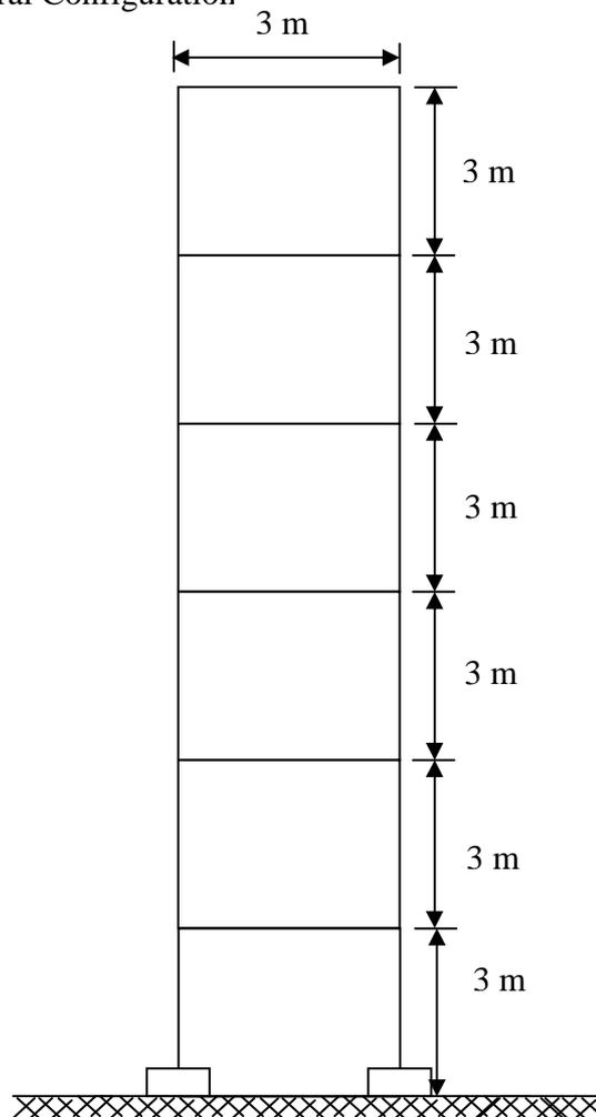
Figure 6.26: Frame to be analyzed by Seismic soil-structure interaction analysis.
