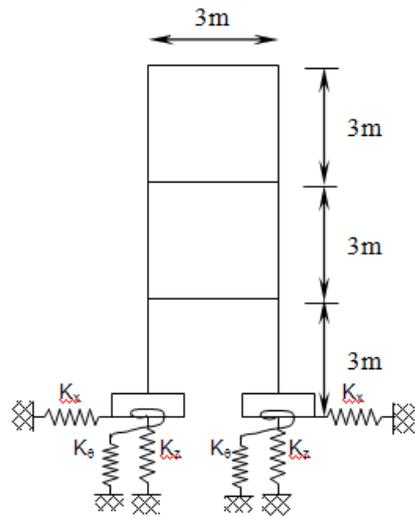
Figure 6.23 : Model of structure only, with spring supports.
