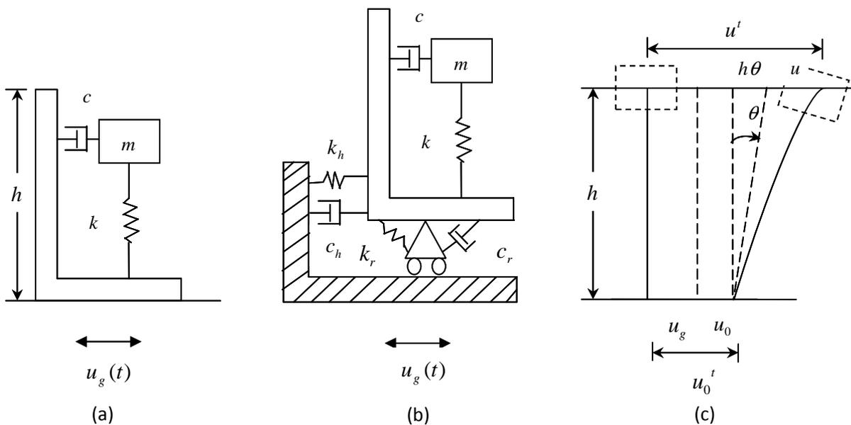
Figure 6.9: Model with compliant base material having one dynamic degree of freedom: (a) SDOF system on a compliant supporting material; (b) idealized discrete system in which the compliance of base is shown by translational and rotational springs and dashpots and (c) total displacements of base and mass.
