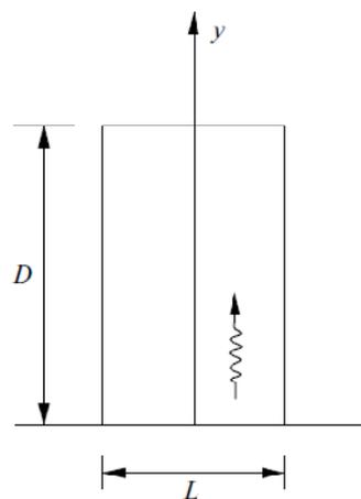
Figure 6.6: Horizontally propagating shear wave in the  $y$ -direction below the rigid slab of a large structure. (Clough and Penzien, 1993)
