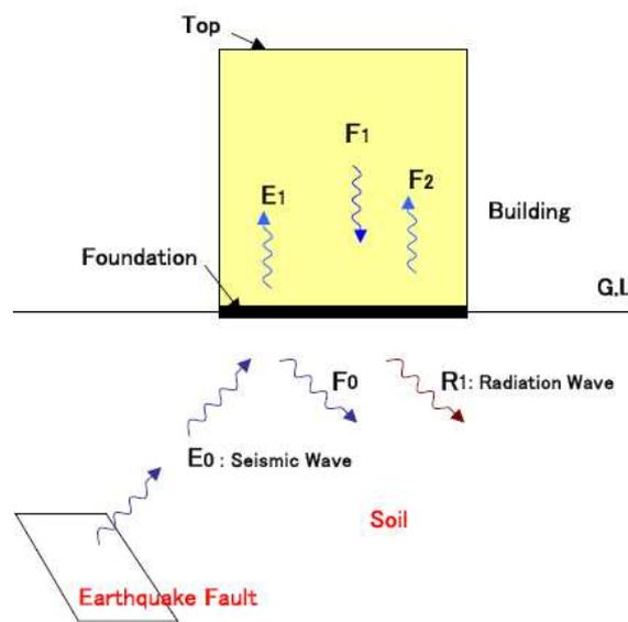
Figure 6.4: Wave propagation during SSI (Miura, 2011)
